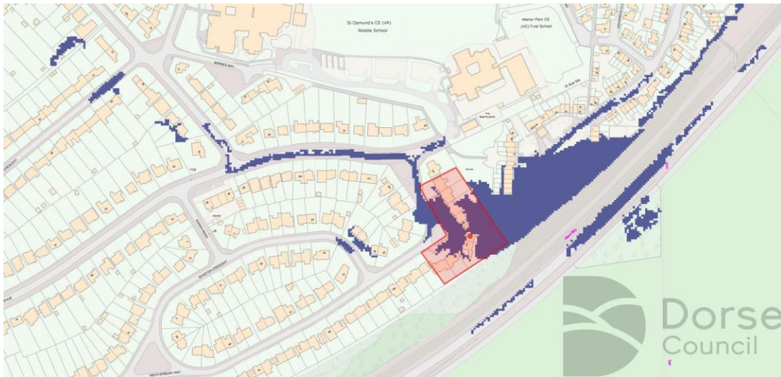
Figure 6 – Surface Water Flood Risk for a 1 in 30 year flood event risk. Weatherbury Way properties in red area
