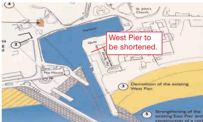
Fig 75. Plan of Harbour Improvement Scheme - construction period 2002 - 2004.
