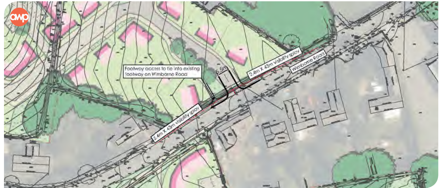
Proposed site access into Sunnyside Farm
