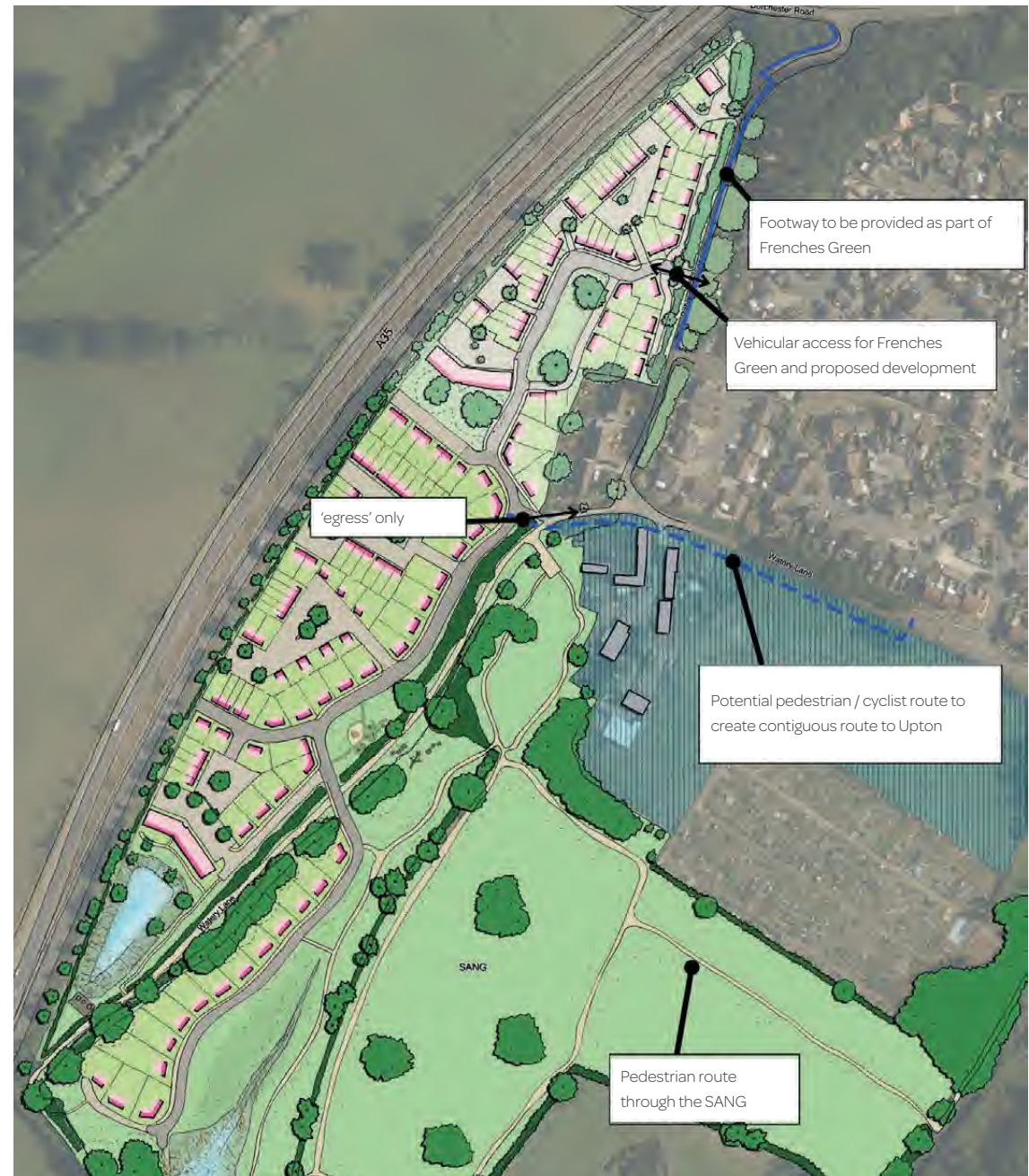
Preliminary site access arrangement and pedestrian routes
